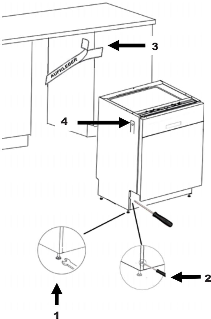
Ensure that the space between the contact surfaces at the top of the appliance is not more than 5 mm. Align the appliance door with the edge of the kitchen furniture unit.
