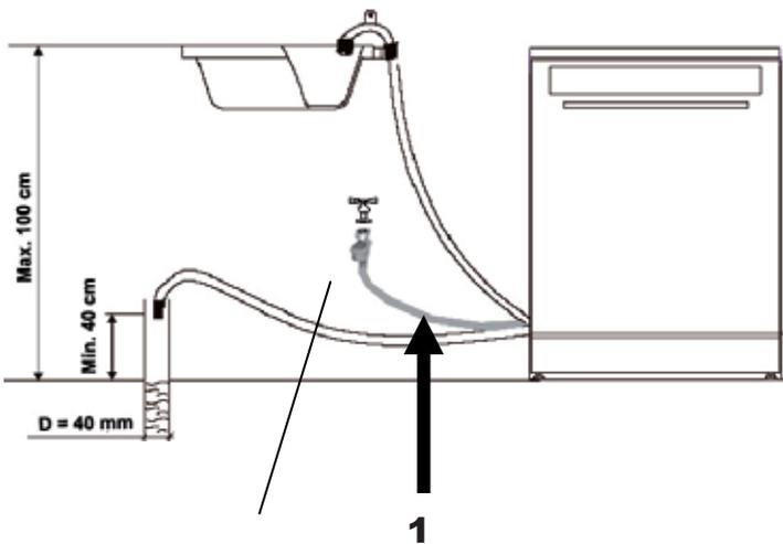
The inlet hose equipped with Aqua-Stop System **1** is provided with double walls.
