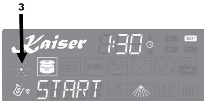
The rinse aid should be added, when the Rinse aid warning light **3** on the information display goes on.
